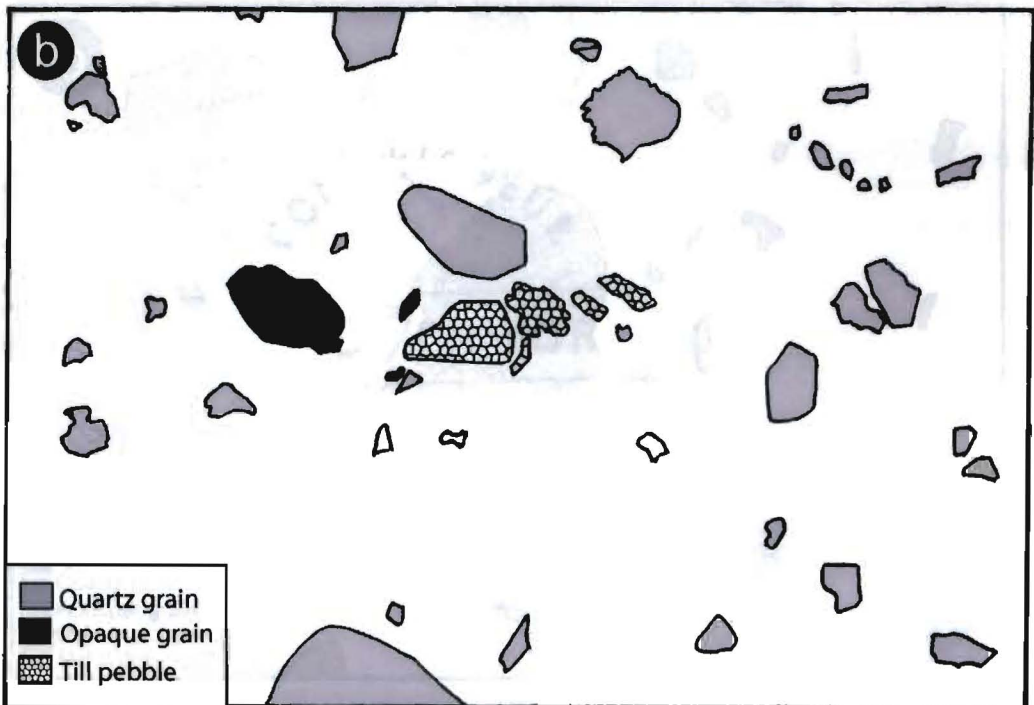
Figure 39 (a, b). Photomicrograph and accompanying sketch of sample 10-02-01. This sample depicts a sheared intraclast (till pebble). Note the juxtaposed grains and their alignment (yellow arrow). Scale bar indicates approximately 1 mm.
