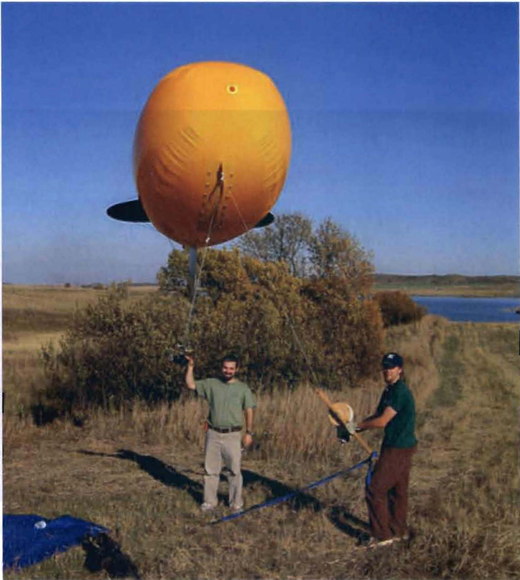
Figure 20. Ground view of author (left) and Shawn Salley (field assistant) holding the helium blimp at Devils Lake Mountain, ND. Helium blimp is 13 ft (4 m) long and lifts the same camera rigs used in kite aerial photography. (Photograph courtesy of James Aber, 2004).
