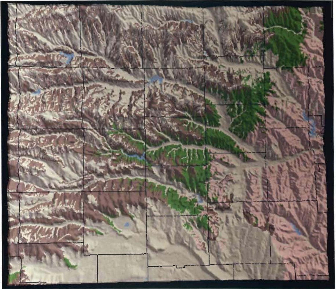
Figure 2: Relationship of Central Kansas Terrain to Generalized Surface Geology. The enhanced shaded relief map depicts the relation of the Dakota Formation (green color) to the surrounding generalized geology (strata below the Dakota are a pink color while strata above the Dakota are a brown color) and sediments (tan color). Lakes/reservoirs are depicted as a blue color. Created from NED and surficial geology GIS datasets downloaded from DASC.
