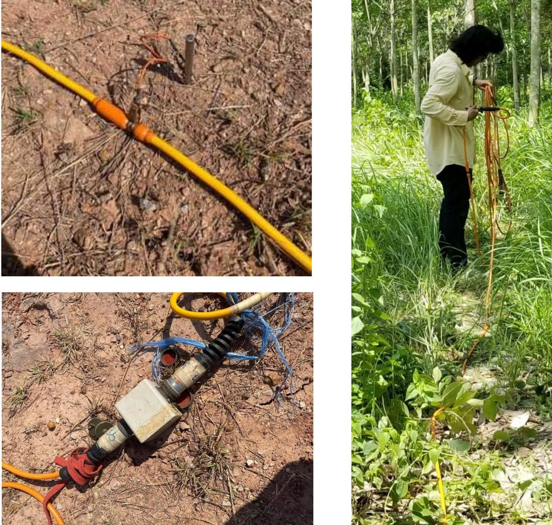
**Figure 3.5** Left (top): cable attached to wire, attached to stainless-steel stake that is inserted into the ground. Left (bottom): ERT electrode. Right: laying ERT survey cable out along the profile. Left photos by Dr. Marcia Schulmeister, right photo by Romyupa Srikraiwest.
