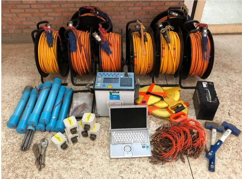
**Figure 3.4** ERT survey equipment includes: a resistivity meter, laptop, cables, electrodes, metal stakes, and multiple tape measures. Photo by Romyupa Srikraiwest.
