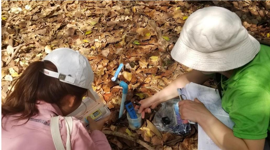
**Figure 3.2** Measuring conductivity with a handheld salinity meter. Photo by Dr. Marcia Schulmeister.
