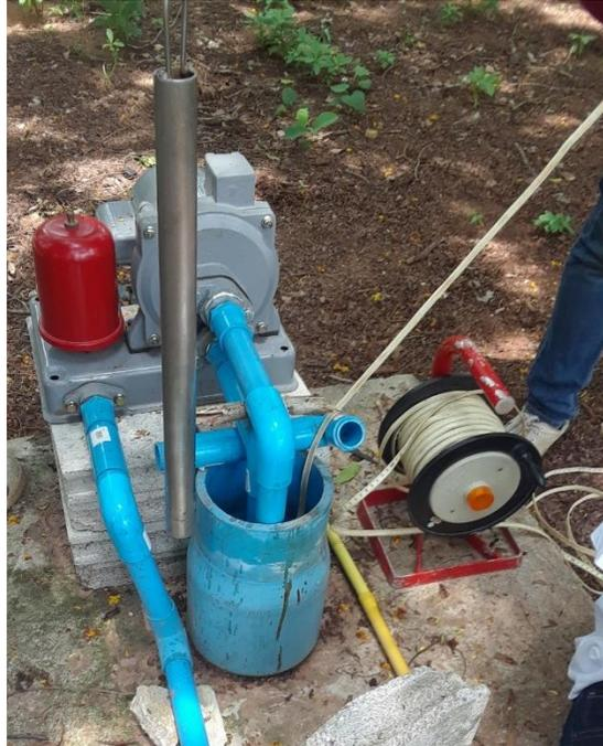
**Figure 3.3** Measuring depth to water in a domestic water well with an electronic tape measure. Photo by Dr. Marcia Schulmeister.
