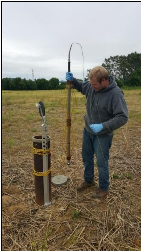
**Figure 4.9** Site photo showing OPTV probe and MW-19 (original).
