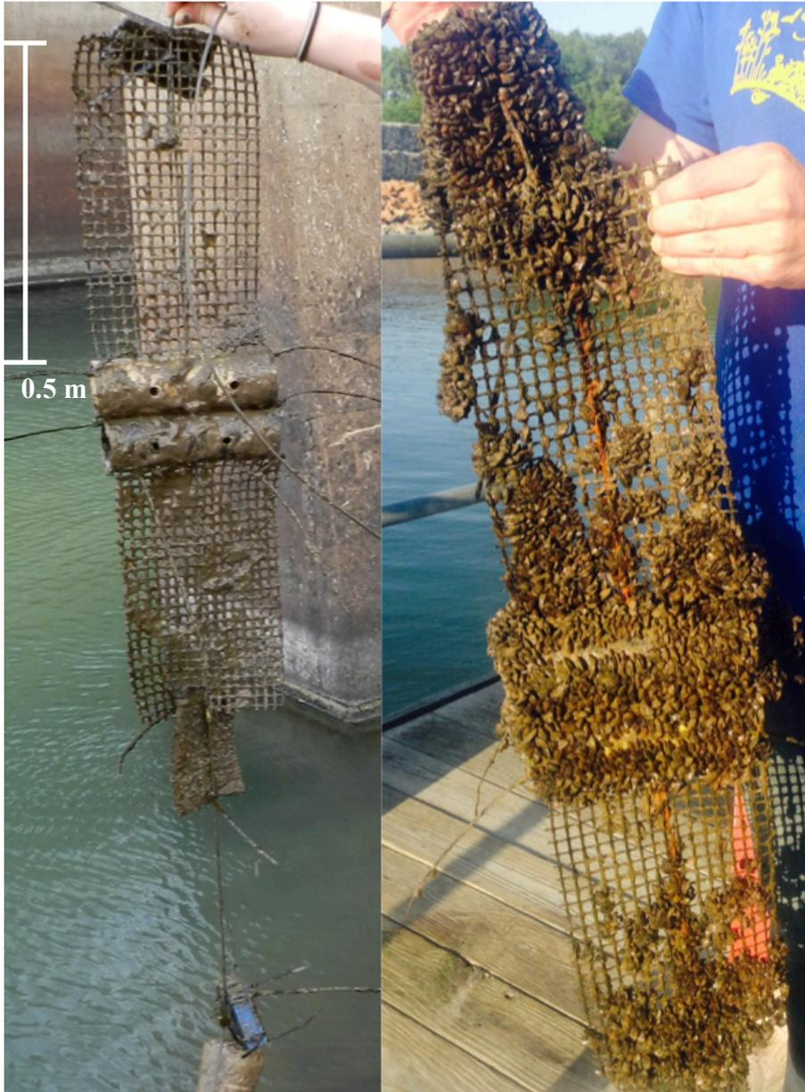
Figure 2. Modified “Portland Sampler” before (left) and after (right) colonization by zebra mussels, deployed at 12 sites in the Marais des Cygnes River and Melvern Lake during 2013–2014.
