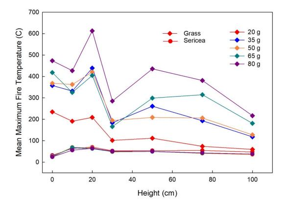
Fig. 1-6. Average max temperature at drying times (24 h, 36 h, and EMC) and varying proportions of sericea (0%, 25%, 50%, 75%, and 100%) at measured heights above the fuel bed (0 cm, 10 cm, 20 cm, 30 cm, 50 cm, 75 cm, and 100 cm).
