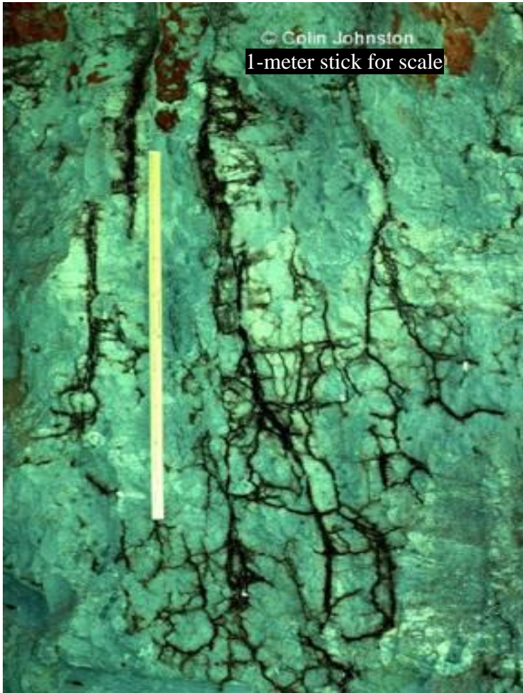
Figure 8. Photograph of fine-grained soil with matrix blocks and dendritic macropore network (Colin Johnston via ITRC, 2013a).
