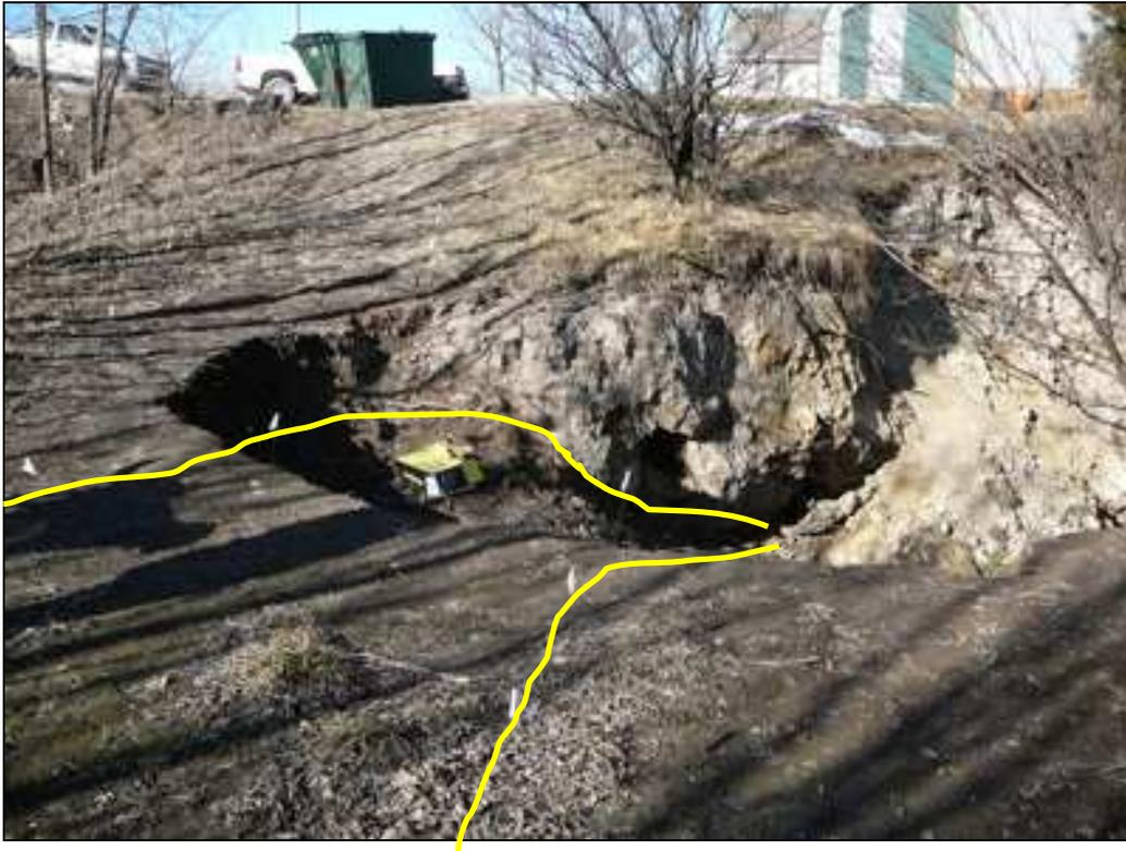
Figure 4.11 Paleosink 1 and Fracture 1 (yellow outline) in 2009. Photo facing north. Note the white pin flags in the lower left corner of the picture that were placed to monitor expansion of Fracture 1.
