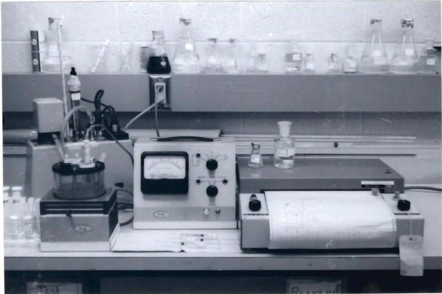
Plate 2: Oxygen polarograph apparatus and recorder.
