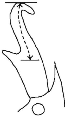
Figure 8. Prong length measurement.
