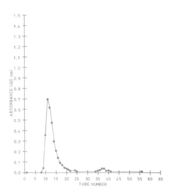
Figure 8. Light absorbance at a wavelength of 420 nm by three fractions of aspergilline inhibited with DMSO at the 70 mM concentration.
