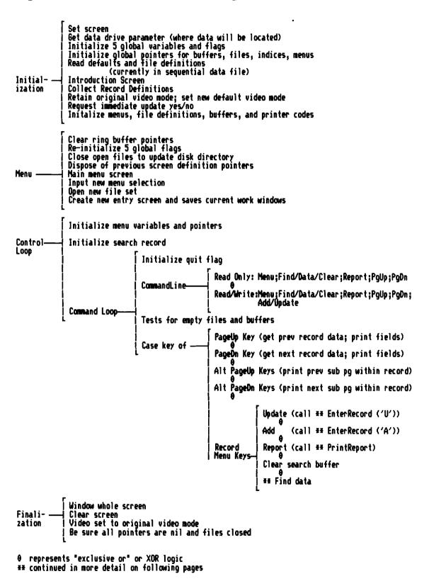
Figure 14: System Structure Diagram (continued)
