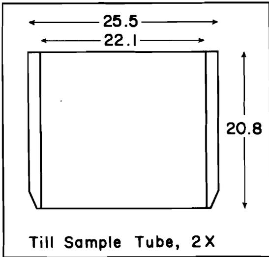
Figure 8. Longitudinal-section diagram of plastic sample tube showing internal and external dimensions in mm. Size of tube was designed to be compatible with laboratory equipment.
