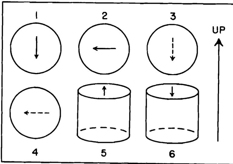
Figure 10. Examples of six-spin sample orientations for spinner magnetometer measurements. A side view of samples as they spin about a vertical axis (up arrow). The small arrow represents the compass orientation on sample top. Based on Collinson (1983, fig. 9.22).
