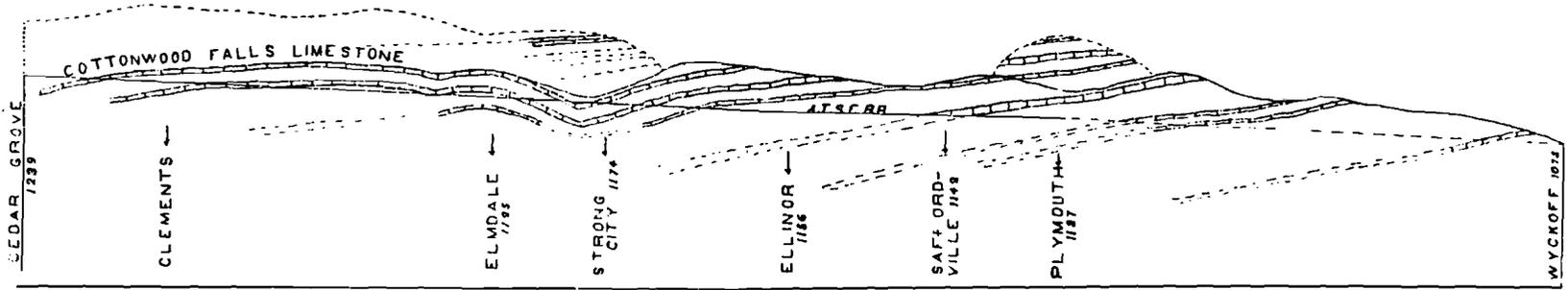
Figure 13. Section of sedimentary rock strata along the Cottonwood River from east of Emporia to southwestern Chase County. Approximate distance from Wyckoff to Cedar Grove (Cedar Point) is 70 km (43 miles). Elevations listed are in feet above sea level. Note the trough at Strong City. Adapted from Kirk in Haworth (1896, plate 3).
