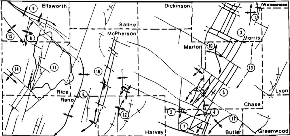
Figure 11. Map showing previously recognized structures in Chase County and surrounding counties. Features of interest in Chase County are: 5. - Cedar Creek syncline, 10. - Elmdale dome, 13. - Humboldt fault. Taken from Berendsen and Blair (1986, figure 3).
