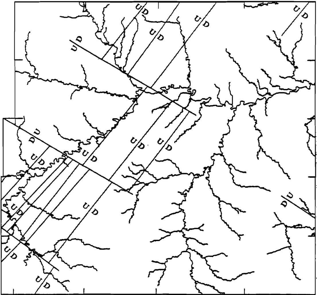
Figure 20. Map of Chase County showing the relationship between the orientations of subsurface fractures in the Arbuckle Group to the orientations of streams. U = upthrown side, D = downthrown side. Fractures in the Ordovician Arbuckle Group are a reflection of even deeper Proterozoic basement fractures. Approximate location and extent of Arbuckle Group fractures taken from Berendsen and Blair (1986, map 6).
