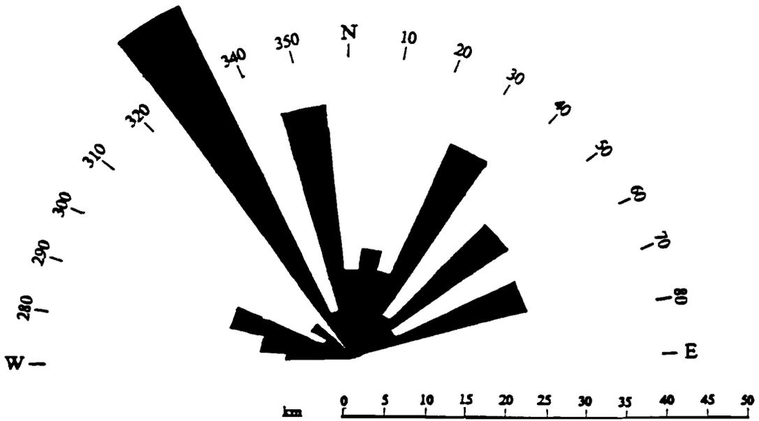
Figure 21. Rose diagram showing the orientations of stream valley lineaments in Chase County. Valley lineaments are classified in  $10^\circ$  intervals. For example, a  $70^\circ$  orientation includes all lineaments between  $65^\circ$  and  $74^\circ$ . Scale indicates the number of kilometers having a specific orientation.
