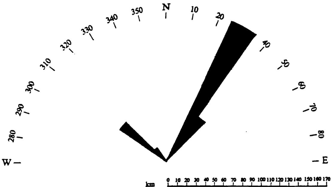
Figure 22. Rose diagram indicating the orientations of subsurface fractures in the Arbuckle Group of Chase County. Fracture data taken from Berendsen and Blair (1986). Scale indicates the number of kilometers of fractures having a certain orientation.
