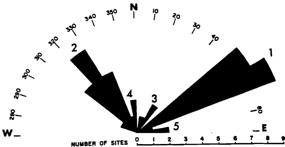
Figure 14. Joint strike orientations for Butler County. Scale indicates number of sites with joints in each 10° interval, and numbers indicate joint sets. Taken from Aber (1992, figure 7).
