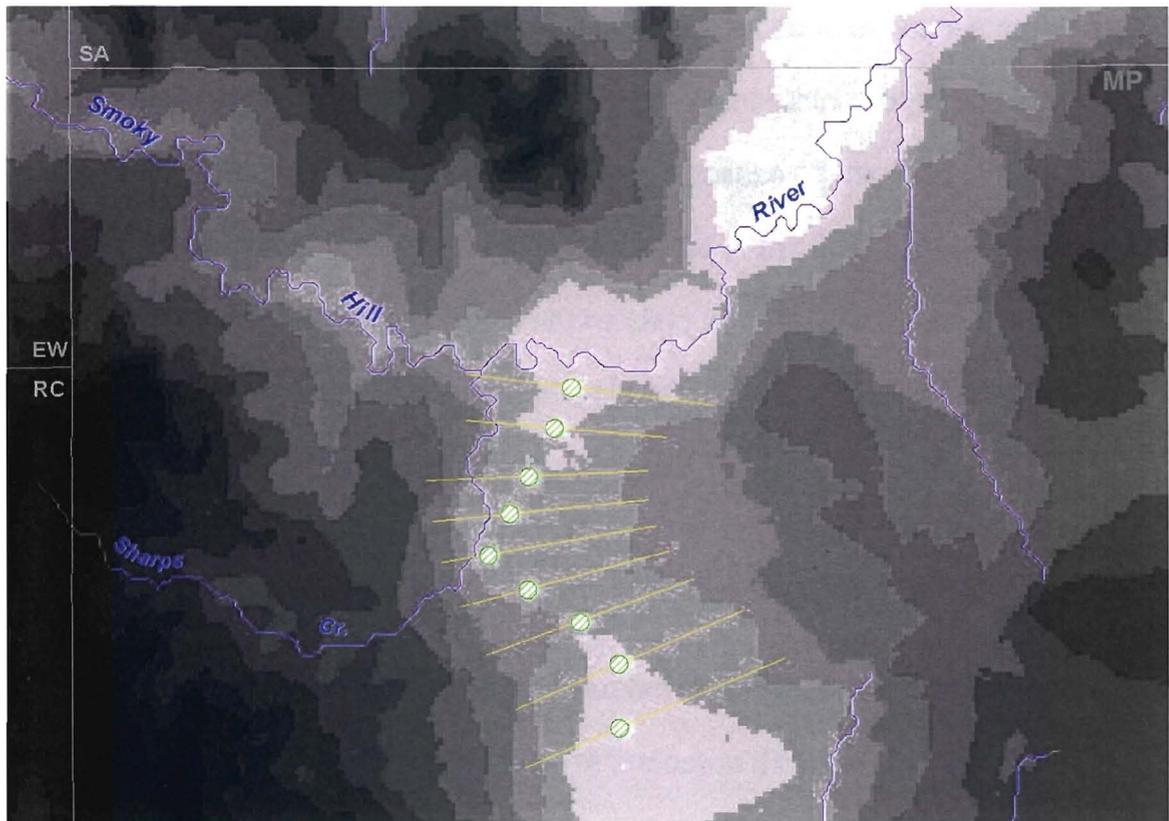
Figure 9. Circular polygons were overlain onto the grid and then summarized to produce the minimum elevation contained within the circle.
