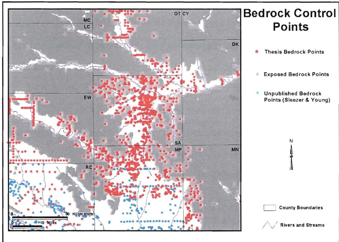
Figure 8. Combined point coverage used to create TIN (Triangulate Irregular Network).
