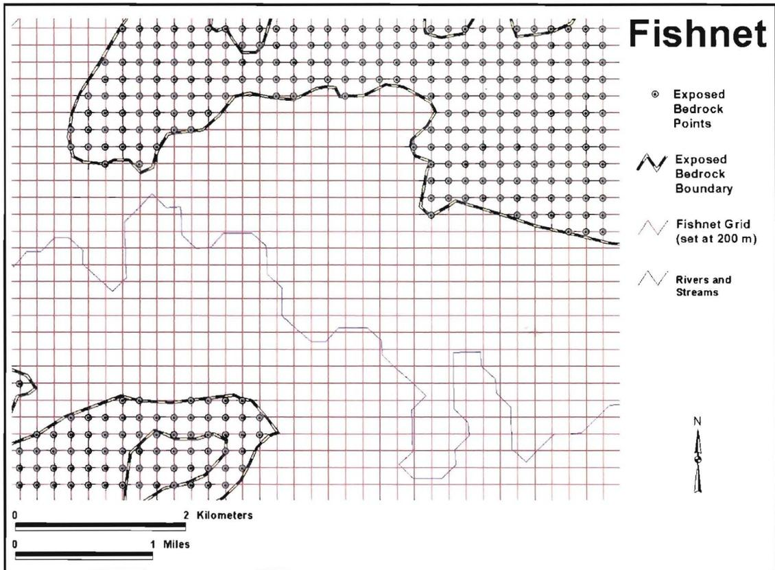
Figure 7. A fishnet was used to figure surface elevation of exposed bedrock. This aided in developing a TIN with less edge effects.
