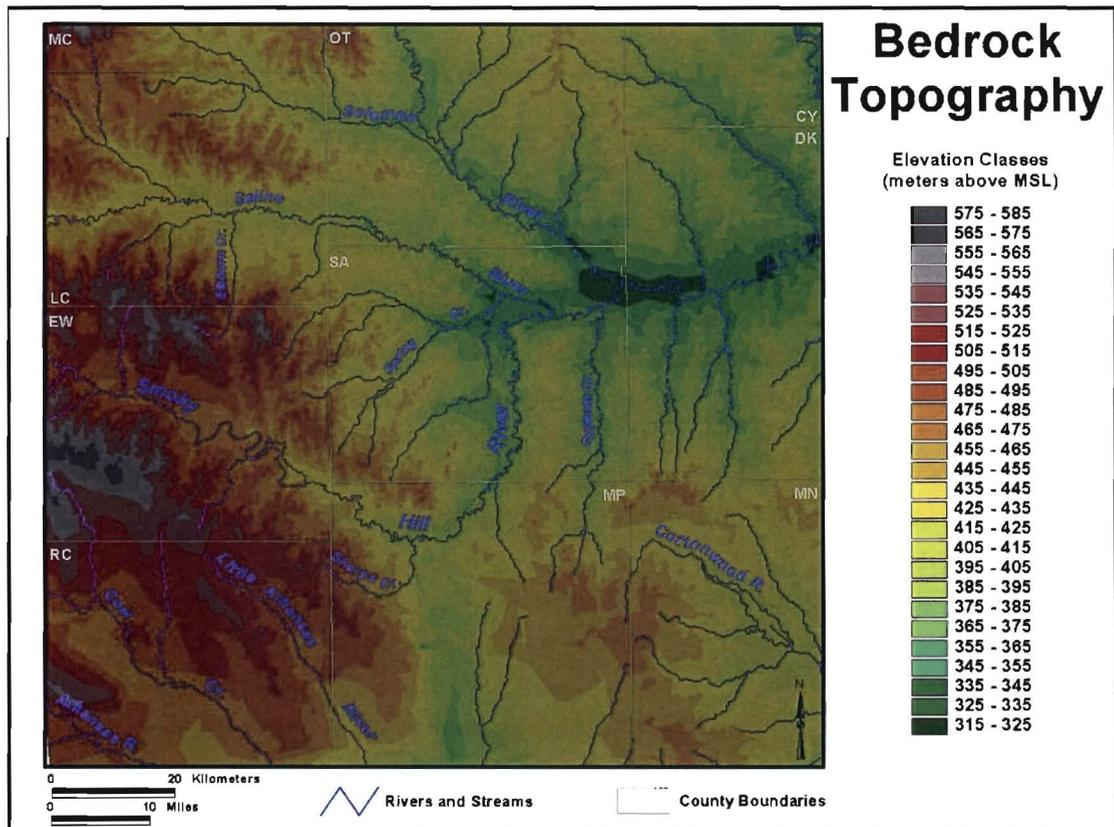
Figure 11. TIN (Triangulated Irregular Network) bedrock topography map created water well logs.
