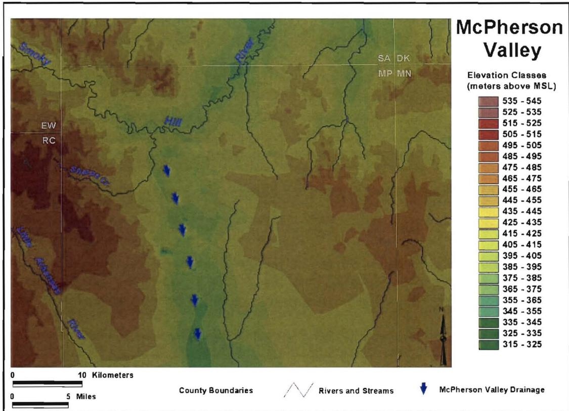
Figure 12. The McPherson Valley paleo-channel in McPherson County, Kansas. The buried channel formed from river incision over soft Permian bedrock.
